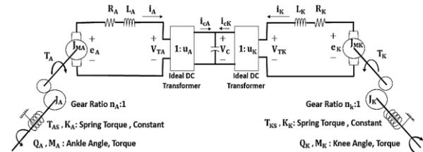
**Figure 1:** Schematic diagram of the electromechanical prosthetic system with motors at ankle (left) and knee (right).
