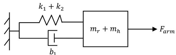
Figure 1: Dynamic model for the power phase.
