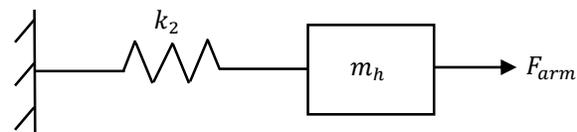
Figure 2: Dynamic model for the recovery phase.
