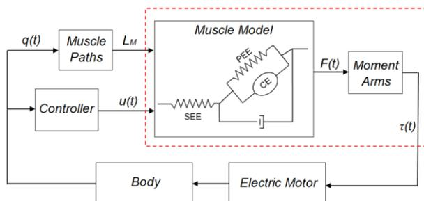
**Figure 1.** Block diagram of the muscle model, in which the red box indicates the scope of this current study
