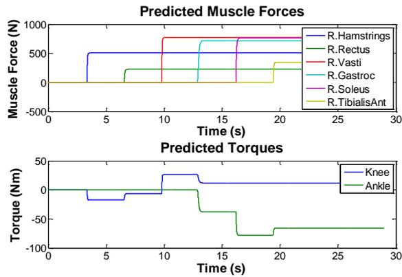
**Figure 2.** Predicted muscle forces (top) and torques (bottom) with constant joint angles  $q(t)$  of zero and step control  $u$
