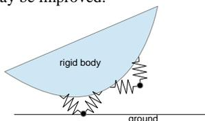
Figure 1: Schematic representation of the contact model.
