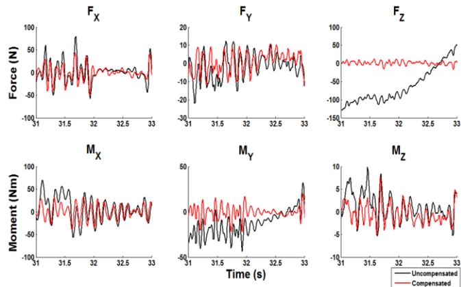
**Figure 1:** Uncompensated (black) and compensated (red) force signals obtained from calibration coefficients of a dissimilar white noise treadmill movements.
