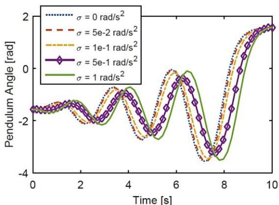
Figure 1 - Optimal trajectories that were found with different noise levels. With increasing noise, the final swing-up occurs later in time.
