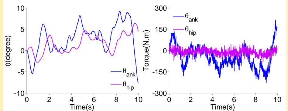
Fig. 3. Example of simulated joint angles (left) and joint torques (right)
