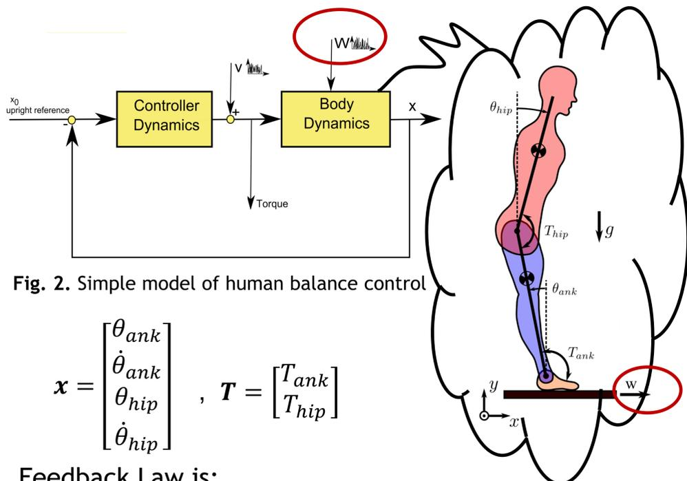
Fig. 2. Simple model of human balance control
