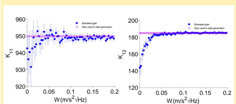
Fig. 4. Estimated feedback gain  $K_{11}$  (left) and  $K_{12}$  (right) for different platform perturbations
