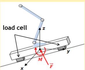
**Figure 1.** Load cells are located underneath both the test subject and the force plate. Inertial errors in ground reaction forces occur when load cells cannot distinguish between the force exhibited by the test subject and the inertia created when the large platform mass is moved
