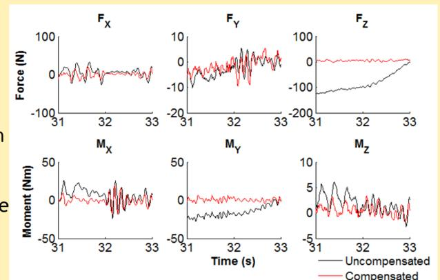
Uncompensated and compensated forces from a moving trial were added to a standard walking trial without platform movement. Results indicate that the compensation method is capable of significantly reducing errors in joint moment calculations that occur when the treadmill platform is moving.
