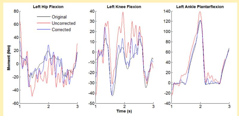
**Figure 3.** Original (black), uncorrected (red), and corrected (blue) joint moments. Errors in hip flexion are reduced from 45% to 17% by implementing the compensation method. The 10% and 20% error in knee and ankle flexion were reduced to 1% and 2%, respectively.
